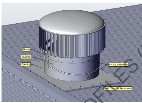
Fix Flashing to roof with 14G Class 3 or 4 Tek screws. Locate 4 close to varipitch and 26 around the 4 sides of the flashing
