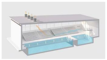
Large spaces with high occupancy usage load are often accompanied by excess heat build-up. In many cases, natural ventilation is not adequate during times of high usage periods. EcoPower allows demand controlled ventilation to significantly increase the rate of extraction. This delivers better airflow control, improved occupant comfort and reduces the load on air conditioning systems
