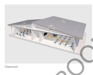
When ducted to the ceiling, EcoPower allows natural ventilation during the day to meet or exceed minimum outdoor air ventilation rates requirements of AS1688.2 and ASHRAE standard 62.1. The powered mode can be activated at night, by a timer or temperature sensor. The night purge operation removes excess heat in the room or building, allowing cool night air to cool the building down. This reduces air conditioning load and lowers energy consumption.
