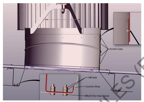
Fix each cyclone fixing strap to the inside of the varipitch with at least 4 x 6-4 AS rivets. Two rivets must be located above the varipitch seam with one through the throat, varipitch and strap.
